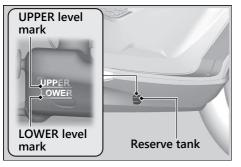
If the coolant level is dropping noticeably or the reserve tank is empty, you likely have a serious leak. Have your vehicle inspected by your dealer.
