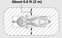
Anyone can unlock the ignition switch and start the engine if your Honda SMART Key is within operating range of your vehicle, even if you are on the other side of a wall or window. If you are away from your vehicle but your Honda SMART Key is still within operating range, deactivate the Honda SMART Key system.
