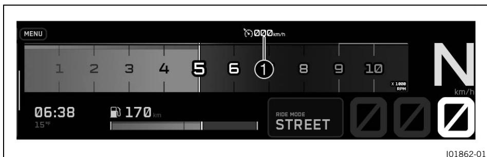
The operating state of the active cruise control is shown in the area ① of the display.
