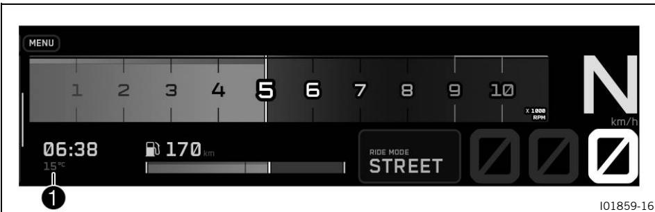
The ambient temperature is shown in area 1 of the display.
