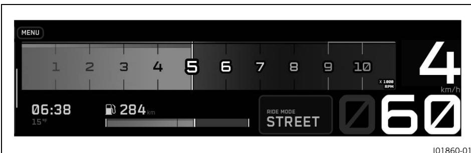
The shift light is integrated in the rpm gauge display.
