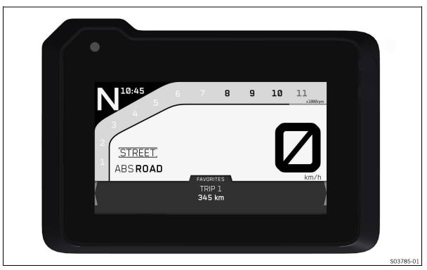
The figure shows the start screen of the combination instrument with the small widget opened. Information can be accessed in the small widget.
