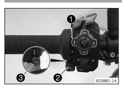
The cruise control buttons ①, ② and ③ of the are located on the left side of the combination switch.
