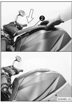
Position fuel tank cover 2 on the fuel tank cap and press it in from the rear to the front.
