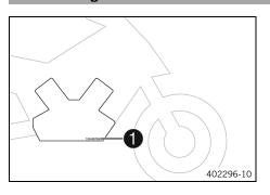
The engine number **1** is stamped on the right side of the engine.
