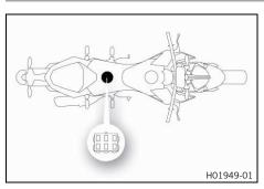
Diagnostics connector 1 is located under the front rider's seat.
