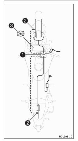
The <u>ABS module</u> ①, which consists of a hydraulic unit, ABS control unit, and return pump, is installed on the right side of the vehicle below the fuel tank. One wheel speed sensor ② is located in each case on the front and the rear wheel.
