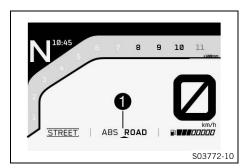
The ABS mode setting is shown in the 1 area of the display. In the menu Motorcycle, the ABS can be configured under ABS Mode.
