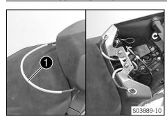
Supporting strap 1 is attached underneath the passenger seat.
