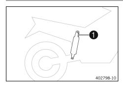
The shock absorber article number **1** is stamped on the top of the shock absorber above the adjusting ring towards the engine side.
