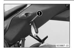
Seat lock is located on the left side of the vehicle under the seat
