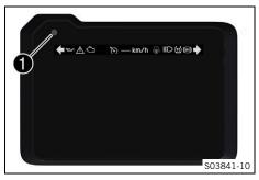
The RACE-ON indicator lamp 1 can indicate errors by flashing. These are indicated up to five seconds after the RACE ON button is actuated.
