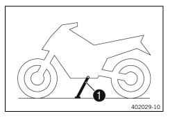
Side stand **1** is located on the left of the vehicle. The side stand is used for parking the motorcycle.
