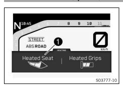
When the seat heating is activated, the **Heated Seat**symbol in area **1** is displayed in the **HEATING** widget.
