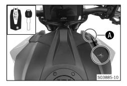
On this vehicle, the ignition/steering lock is replaced by a remote key with transponder (RACE-ON key ( $\mathbb{Q}$  p. 22)).
