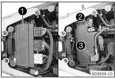
Connect a battery charger to the 12-V battery. Connect the battery charger to the mains connection.
