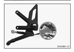
Separate the shift linkage from the shift lever and mount in position "R".
