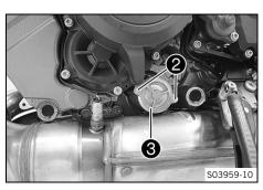
Remove 2 screws. Take off oil filter cover 3 with the O-ring.
