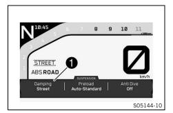
The **Damping** mode setting is shown in the **1** area of the display. The damping can be configured in the **Motorcycle** menu under **Damping**.
