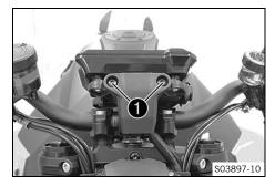
Position the cover, mount and tighten screws 1.
