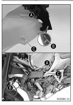
Position the fuel tank spoiler on holding lugs (A), (B) and (C) and slide from front to rear.
