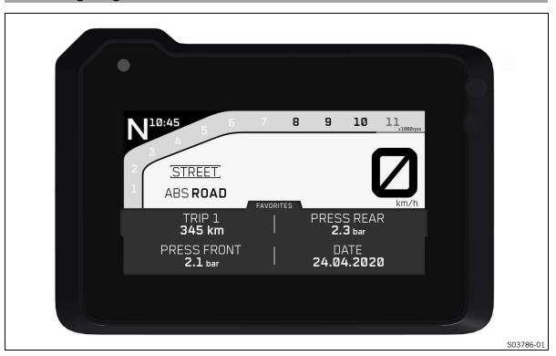
The figure shows the start screen of the combination instrument with the large widget opened. Information can be accessed and configured in the large widget.
