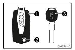
In this vehicle, the RACE-ON key  $\bigcirc$  performs all the functions of the conventional ignition key.
