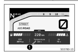
The large **INFO** widget displays the ambient air temperature in area **①**.
