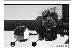
The **+RES** button **1** is fitted on the handlebar, front left. The **-SET** button **2** is fitted on the handlebar, rear left.
