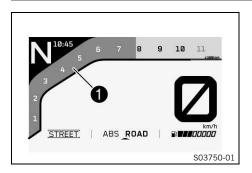
The engine speed is shown in area **1** of the display. The engine speed is measured in revolutions per minute.
