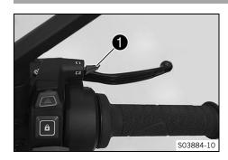
The C1 and C2 switch is fitted on the right of the combination switch.
