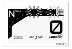
The shift warning light is integrated in the tachometer display. In the **Settings** menu under **Shift Light**, the engine speed for the shift warning light can be set. The shift warning light is always active during the running-in phase (up to 1,000 km / 621 mi). The shift warning light can only be deactivated, and the values for **RPM 1** and **RPM 2** can only be adjusted after this. The shift warning light flashes slowly at **RPM 1** and flashes quickly at **RPM 2**.
