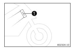
The vehicle identification number **1** is stamped on the right side of the steering head.
