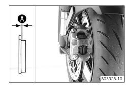
Check all brake linings on both brake calipers for their lining thickness (A).
