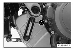
Add the engine oil to upper marking A on the engine oil level viewer
