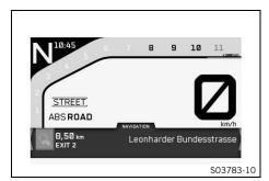
The direction arrow, the distance to the next waypoint and the street name are displayed in the small **NAVIGATION** widget when the navigation function is activated.
