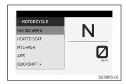
The motorcycle traction control (<u>cornering MTC</u>) lowers the engine torque in case of loss of traction in the rear wheel.
