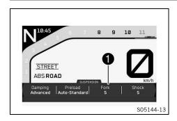
In the **SUSPENSION** widget of the display, the setting of the fork damping is displayed in the **1** area.
