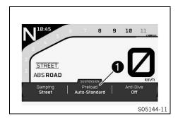
The payload setting is shown in area of the display. The payload can be configured in the **Motorcycle** menu under **Load**.
