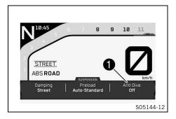
In the **SUSPENSION** widget of the display, the **Anti Dive** mode is displayed in the **1** area.
