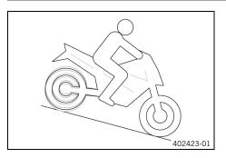
The <u>MSR</u> is an optional auxiliary function of the engine control. If the engine braking effect is too great, the **MSR** prevents the rear wheel from locking or sliding away on a sloping position.
