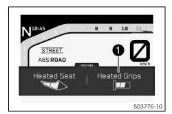
When the heated grip is activated, the **Heated Grips**symbol in area 1 is displayed in the **HEATING** widget.
