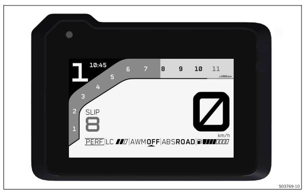
The figure shows the start screen of the combination instrument in active drive mode TRACK (optional) in the performance layout.
