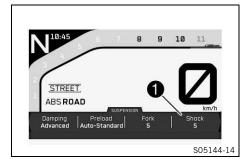
In the **SUSPENSION** widget of the display, the setting of the shock absorber damping is displayed in the **1** area.
