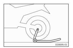
Place the adapter into the rear lifting gear.
