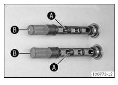
Thoroughly clean magnets **A** and oil screens **B** of the oil drain plugs.
