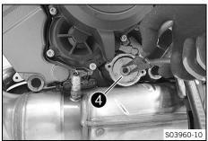
Pull oil filter 4 out of the oil filter housing.
