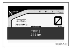
The odometer can be displayed in the **FAVORITES** widget as **Trip 1**. To do this, the information must be configured in the widget. Information on the total distance covered can be accessed in the **General Info** menu under menu item **ODO** or configured as widget information.
