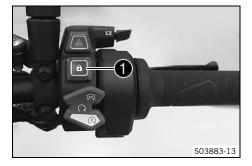
The <u>RACE-ON button</u> **1** is fitted on the right side of the combination switch.
