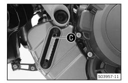
Remove the filler plug with the O-ring and add the second partial quantity up to the upper marking on the engine oil level viewer.
