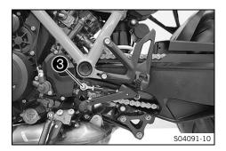
Position the shift linkage at one of the upper positions of the shift shaft.
