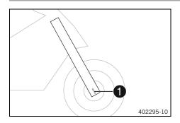
The fork part number **1** is stamped on the inside of the axle clamp.
