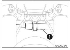
Steering damper item number **1** is embossed on the underside of the steering damper.
