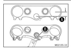
On this vehicle, the handling characteristics can be influenced by the fork offset.
