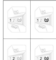
The combination switch displays the current riding mode and traction control setting.
