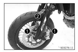
Position the left fork protector. Mount and tighten screws ①.
