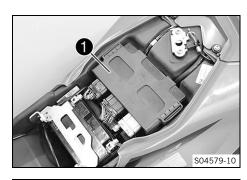
Remove a defective main fuse 3 with needle nose pliers.
