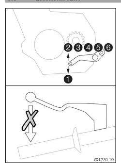
If the QUICKSHIFTER+ is activated, you can shift up and down without actuating the clutch.
