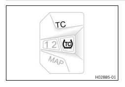
The motorcycle traction control (<u>cornering MTC</u>) lowers the engine torque in case of loss of traction in the rear wheel. Depending on the riding mode, different amounts of slip are allowed when the traction control is activated.
