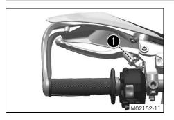
Adjust basic position of the clutch lever to your hand size by turning adjusting screw ①.
