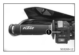
The turn signal switch **1** is fitted on the left side of the handle-
