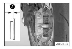
Check the brake linings for lining thickness **A**.
