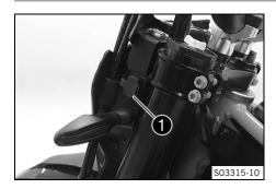
A USB socket **1** for supplying power to external devices is located on the left side of the headlight mask.
