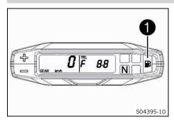
When the fuel level has reached the reserve mark, **TR1 F** appears on the display, and the fuel level warning lamp lights up. This indicator can be closed by pressing the + or - button.
