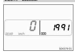
Press the + or - button repeatedly until **000** is shown on the combination instrument.
