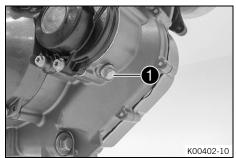
Mount and tighten screw with a new seal ring.
