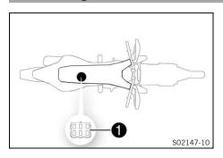
Diagnostics connector 1 is located under the engine control unit.
