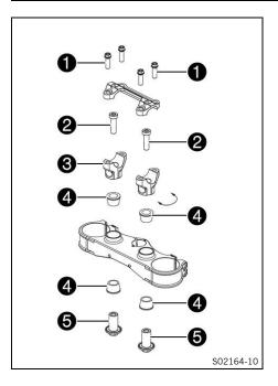
Remove screws 1. Take off the handlebar clamp. Remove the handlebar and lay it to one side.
