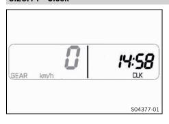
Press the + or - button repeatedly until CLK is shown on the combination instrument.
