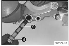
Remove screw plug 8 with oil screen 9 and the O-rings.
