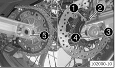
Push the rear wheel forward as far as possible and take the chain off the rear sprocket.
