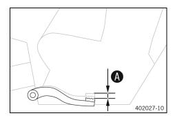
Move the foot brake lever back and forth between the end stop and the contact to the foot brake cylinder piston and check free travel A.
