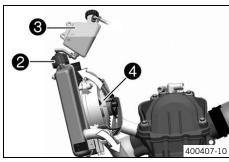
The coolant is cooled by the air stream and radiator fan **4**, which is activated depending on the temperature.
