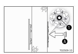
Clean and grease the thread of the wheel spindle and nut 2.
