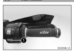
Start button 1 is fitted on the right side of the handlebar.
