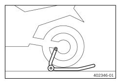
Insert the adapter in the rear of the lifting gear and screw into the link fork on both sides.
