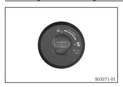
The ignition and steering lock is located in front of the seat.
