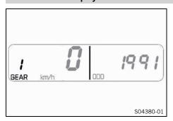
The gear display shows the engaged gear.
