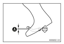
Sit on the vehicle in the riding position and determine distance A between the upper edge of your boot and the shift
