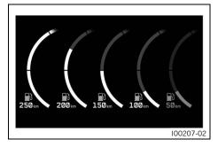
The fuel level display consists of the fuel range display and a bar. The higher the bar is filled, the more fuel is in the fuel tank
