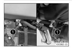
A fuel cock 1 is located on each side of the fuel tank.
