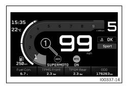
The ABS mode setting is shown in the **1** area of the display. When the **Ride Mode Track** ( p. 134) is activated, the ABS can be configured in the **ABS** submenu.
