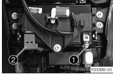
Connect a battery charger to the 12-V battery. Connect the battery charger to the mains connection.
