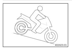
The <u>MSR</u> is an optional auxiliary function of the engine control. If the engine braking effect is too great, the **MSR** prevents the rear wheel from locking or sliding away on a sloping position.
