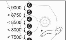
If the QUICKSHIFTER+ (optional) is activated in the combination instrument, you can shift down in the speed range shown without pulling the clutch lever.
