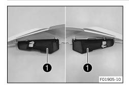
The left or right storage compartment contains the on-board tool set  $\bigcirc$ .
