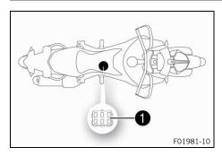
Diagnostics connector 1 is located under the battery cover.
