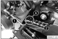
Position T-wrench 1 in area A between the chain and chain sliding guard 2.
