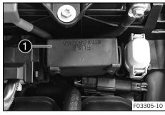
Remove the faulty fuse.
