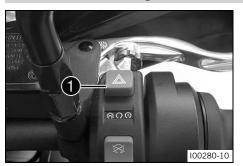
The hazard warning flasher switch **1** is fitted on the right side of the switch.
