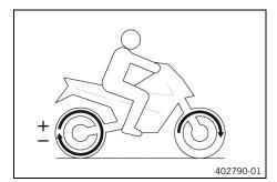
The spin adjuster is a motorcycle traction control function. The slip adjustment allows the motorcycle traction control to be tuned through nine levels to the desired characteristic map. Level 1 allows the maximum slip on the rear wheel, and level 9 the minimum.
