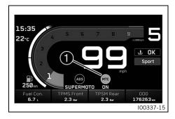
The  $\bigcirc$  area of the display indicates whether  $\underline{\text{MTC}}$  ( $\bigcirc$  p. 134) is switched on or off.
