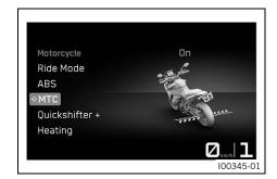
The motorcycle traction control ( $\underline{MTC}$ ) lowers the engine torque in case of loss of traction in the rear wheel. Depending on the riding mode ( $\underline{\blacksquare}$  p. 134), different amounts of slip are allowed when traction control is activated.
