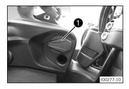
Socket **1** for electrical accessories is mounted on the left side of the mask support.
