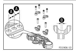
On the upper triple clamp, there are three holes at a distance of  $\bf A$  to each other.
