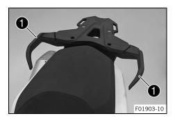
The grab handles **①** are used for moving the motorcycle around. If you carry a passenger, the passenger can hold onto the grab handles during the trip.
