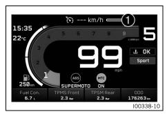
The operating state of the active cruise control is shown in the area
