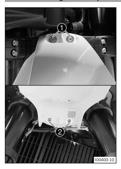
Remove screws 1 and 2. Take off the front fender.
