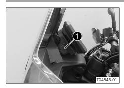
USB socket **1** for the power supply to external devices is mounted on the left side of the mask support.
