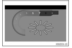
The shift light is integrated in the rpm gauge display. In the **Shift Light** submenu, the engine speed for the shift warning light can be set. The shift warning light is always active during the running-in time (up to 1000 km / 621 mi). The shift warning light can only be deactivated, and the values for **RPM1** and **RPM2** can only be adjusted after this. At **RPM1**, the engine speed display flashes red and at **RPM2**, the entire display flashes red.
