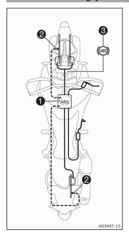
The <u>ABS</u> module ①, which consists of a hydraulic unit, ABS control unit, and return pump, is installed under the fuel tank. One wheel speed sensor ② is located in each case on the front and the rear wheel.
