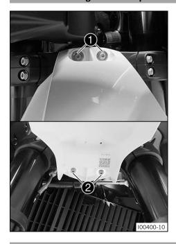
Position the front fender. Mount and tighten screws 1
