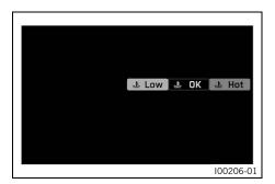
The coolant temperature is displayed by a symbol. The symbol changes between **LOW**, **OK** and **HOT** depending on the temperature.
