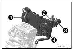
The coolant is cooled by the air stream and two radiator fans **4**, which are activated at high temperature.
