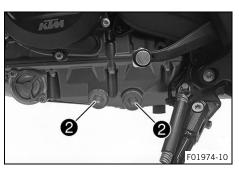
Remove oil drain plugs 2 along with the magnets, the O-rings, and the oil screens.
