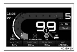
The status of the grip heater is shown in area **1** of the display. The grip heater can be configured in the **Heated Grip** menu.
