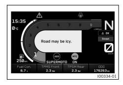
The ice warning \*appears on the display when the ambient temperature drops below the specified value.
