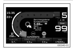
The **Navigation** indicator appears when the navigation function is activated.
