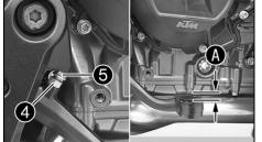
Loosen nut 4 and turn screw 5 correspondingly until the free travel A is present. If necessary, adjust the basic position of the foot brake lever.
