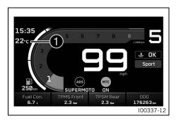
The ambient temperature is shown in area **1** of the display. The ambient air temperature is displayed in **°C** or **°F**.
