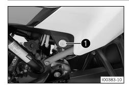
Seat lock 1 is located on the left side of the vehicle. It can be unlocked using the ignition key.
