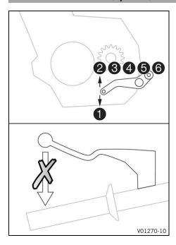
If the QUICKSHIFTER+ is activated, you can shift up and down without actuating the clutch.
