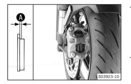
Check all brake linings on both brake calipers for their lining thickness (A).
