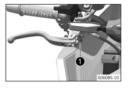
Push the hand brake lever forward.
