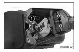
The tool set **1** is located under the passenger seat.
