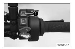
The hazard warning flasher switch **1** is fitted on the right side of the combination switch.
