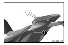
The ① tip switch of the passenger seat release is located on the left side of the vehicle below the passenger seat. The passenger seat release tip switch only functions if the motor-cycle is stationary, the engine is switched off and the ignition is switched on or switched off for less than 1 minute. If the passenger seat release tip switch does not work, the passenger seat can be unlocked using the passenger seat emergency release (I p. 25).
