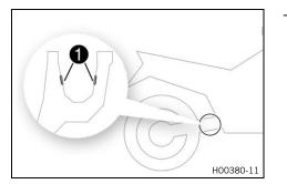
If the protection caps are damaged or loose: - Replace the protection caps.
