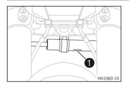
Steering damper item number **1** is embossed on the underside of the steering damper.
