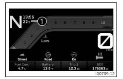
The ambient temperature is shown in area ① of the display. The ambient air temperature is displayed in °C or °F. The unit of the ambient air temperature can be configured in the **Temperature** submenu.
