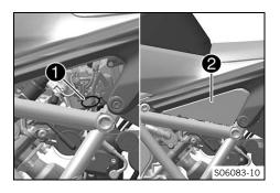
The passenger seat emergency release ① is located on the left side of the vehicle below the ② cover. The emergency passenger seat release is used if the seat release
