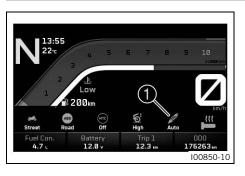
The **Damping** mode setting is shown in the **①** area of the display. The damping can be configured in the **Suspension** menu under **Damping**.
