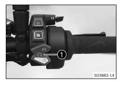
The start button/emergency OFF switch 1 is fitted on the right side of the combination switch.
