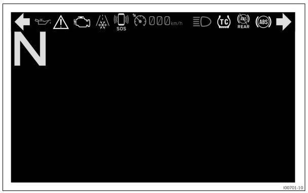
The indicator lamps offer additional information about the operating state of the motorcycle. When the ignition is switched on, all indicator lamps light up briefly, except for the TC indicator lamp .
