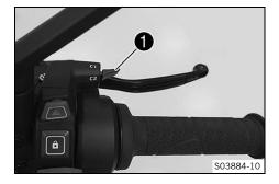
The C1 and C2 switch is fitted on the right of the combination switch.
