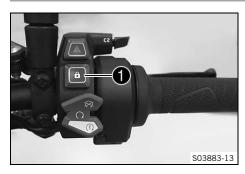
The Unlock button 1 is fitted on the right side of the combination switch.
