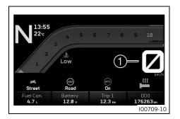
The speed is shown in area ① of the display. Speed is shown in kilometers per hour **km/h** or in miles per hour **mph**. The unit of speed can be configured in the **Distance** submenu.
