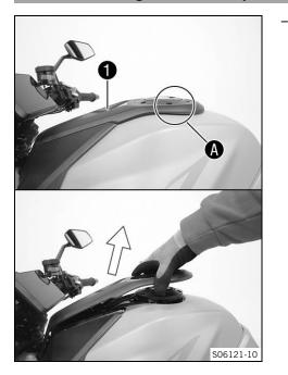
Raise fuel tank cover **1** in area **A** and remove in the upward direction.
