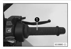
The throttle grip lacksquare is fitted on the right side of the handlebar.
