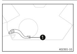
Foot brake lever **1** is located in front of the right footrest. The rear brake is engaged with the foot brake lever.
