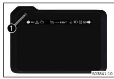
The RACE-ON indicator lamp ① can indicate errors by flashing. These are indicated up to five seconds after the RACE ON button is actuated.
