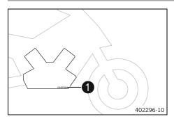
The engine number **1** is stamped on the right side of the engine.
