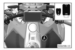
On this vehicle, the ignition and steering lock is replaced by a with transponder key (RACE ON key (I p. 22)).
