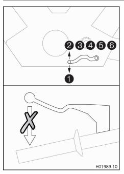
If the <u>QUICKSHIFTER+</u> (optional) is activated, you can shift up and down without actuating the clutch.
