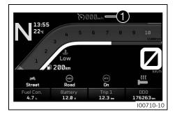
The operating state of the active cruise control is shown in the area  $\bigcirc$  of the display.
