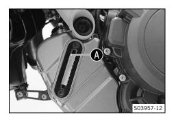
Add the engine oil to upper marking  $oldsymbol{A}$  on the engine oil level viewer.
