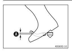
Sit on the vehicle in the riding position and measure the distance A between the upper edge of your boot and the shift lever.
