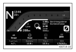
Pressing the **C1** or **C2** button calls up the configured menu. Press the **BACK** button to close the **Custom Switch** display.
