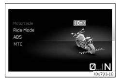
The motorcycle traction control (<u>MTC</u>) (optional) lowers the engine torque in case of loss of traction in the rear wheel. Depending on the <u>riding mode</u> ( $\square$  p. 138), different amounts of slip are allowed when traction control is activated.
