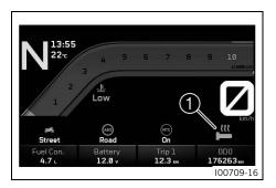
The status of the heated grip is shown in area **①** of the display. The heated grip can be configured in the **Heated Grip** menu.
