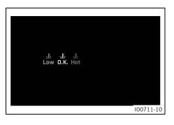
The coolant temperature is displayed by a symbol. The symbol changes between **LOW**, **OK** and **HOT** depending on the temperature.
