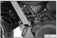
Mount and tighten oil drain plugs ① with magnets, O-rings, and oil screens.
