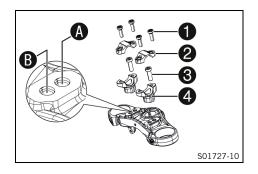
Remove screws **1**. Take off the handlebar clamps **2**. Position the handlebar so that screws **3** are accessible.
