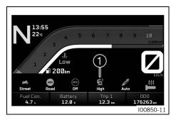
The payload setting is shown in area ① of the display. The payload can be configured in the **Suspension** menu under **Load**.
