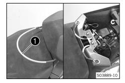
Supporting strap **1** is attached underneath the passenger seat.
