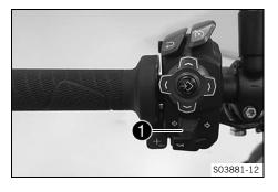
Turn signal switch ① is fitted on the combination switch on the left.
