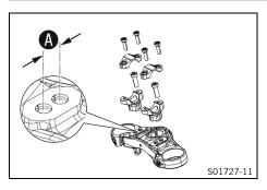
On the upper triple clamp there are two holes at a distance of A apart.
