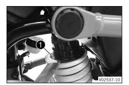
Adjust the spring preload by turning adjusting ring using the hook wrench from the tool set.
