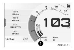
The ABS mode setting is shown in the **1** area of the display. The ABS can be configured in the **ABS** submenu.
