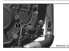
Water pump **1** in the engine ensures forced circulation of the coolant.
