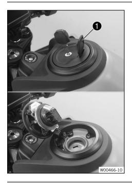
Lift cover **1** of the fuel tank filler cap and insert the ignition key into the lock.
