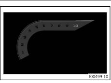
The engine speed is displayed in revolutions per minute.
