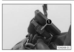
USB socket ① for the power supply to external devices is mounted on the left side of the mask support. The USB socket is activated when the ignition is switched on.
