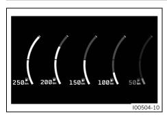
The fuel level display consists of the fuel range display and a bar. The higher the bar is filled, the more fuel is in the fuel tank
