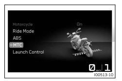
The motorcycle traction control (MTC) (optional) lowers the engine torque in case of loss of traction in the rear wheel. Depending on the riding mode (E p. 106), different amounts of slip are allowed when traction control is activated.
