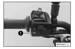
Horn button **()** is fitted on the left side of the handlebar.
