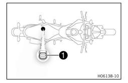
Diagnostics connector **1** is located under the seat.
