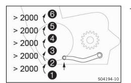
If the <u>QUICKSHIFTER+</u> (optional) is activated in the combination instrument, you can shift up in the engine speed range indicated without pulling the clutch lever.
