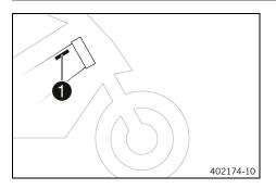
The type label 1 is on the right of the frame behind the steering head.
