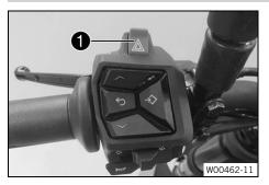
The hazard warning flasher switch ① is fitted on the top of the combination switch.
