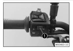
Turn signal switch **1** is fitted on the left side of the handlebar. **Possible states**
