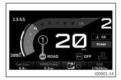
The ABS mode setting is shown in the **①** area of the display. ABS can be configured separately in the **ABS** submenu.
