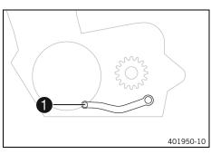
Shift lever **1** is mounted on the left side of the engine.
