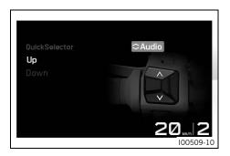
When the menu is closed, the  ${\bf Quick\ Selector\ 1}$  display is opened by pressing the  ${\bf UP}$  button.
