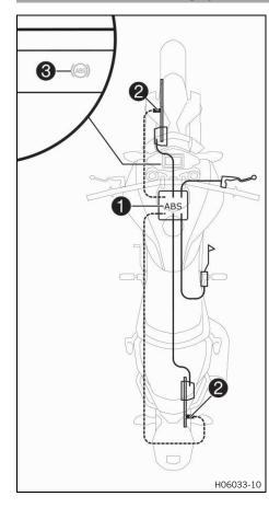
The <u>ABS</u> module **①**, which consists of a hydraulic unit, ABS control unit, and return pump, is installed under the fuel tank. One wheel speed sensor **②** is located in each case on the front and the rear wheel.
