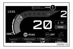
The operating status of the activated speed limiter is shown in display area **1**.
