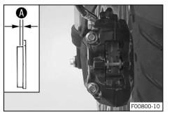
Check the brake linings for lining thickness (A).
