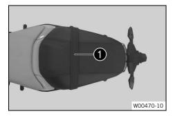
Supporting strap ① is used for maneuvering the motorcycle. If you carry a passenger, the passenger can hold onto the grab handles during the trip.
