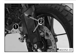
Position the fork protector. Mount screw 1 with the reflector, but do not tighten yet.
