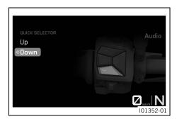
When the menu is closed, the  $\bf Quick\ Selector\ 2$  display is opened by pressing the  $\bf DOWN$  button.
