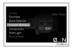
Pressing the **C** button calls up the configured menu. Press the **BACK** button to close the **Custom Switch** display.
