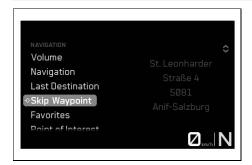
Condition: Function **Bluetooth®** activated, **KTMconnect** app (optional) is installed and opened on a suitable cell phone, The dashboard is connected to a suitable cell phone, GPS function is activated on the connected cell phone, Navigation with at least one interim destination has been started in the **KTMconnect** app (optional)
