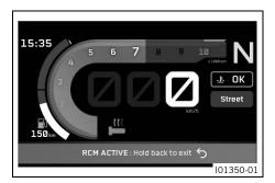
The Remote Control Mode indicator (optional) appears when Remote Control Mode is activated.
