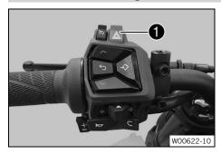
The hazard warning flasher switch **1** is fitted on the top of the combination switch.
