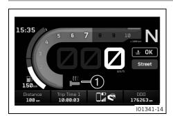
The status of the heated grip is shown in area of the display. The heated grip can be configured in the **Heated Grips** menu.
