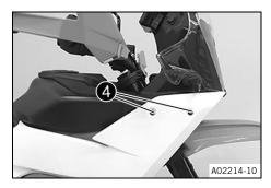
Mount and tighten screws 4.
