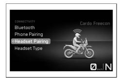
Condition: Motorcycle is stationary, Function **Bluetooth®** activated, Function **Bluetooth®** also activated on the device that is to be paired
