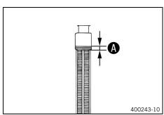
Pour coolant in up to level above the radiator fins.
