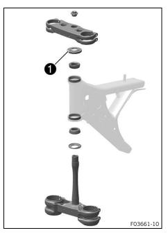
Clean the bearing and sealing elements, check for damage, and grease.
