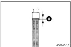
Pour coolant in up to level above the radiator fins.
