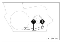
Remove screw with the washers and take off shift lever 2.
