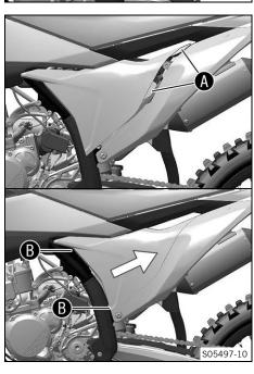
The air filter box cover is not secured.
