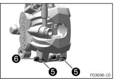
Insert the new brake linings, insert pin 6, and mount cotter pins 5.
