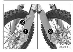
Position the fork protection on the left fork leg. Mount and tighten screws 1.
