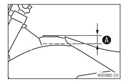
Fill the fuel tank with fuel up to measurement A.
