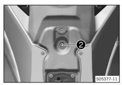
Mount and tighten screw ② with the rubber bushing.
