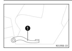
Foot brake lever **1** is located in front of the right footrest.
