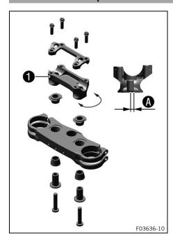
The holes on the handlebar support **1** are placed at a distance of **A** from the center.
