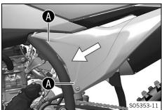
Pull off the air filter box cover in area **A** and push it sideways and forward. Take off the air filter box cover.
