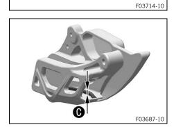
Check the chain guide with a slide gage for dimension **()**.
