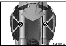
Remove screws 6 with the collar bushings.
