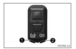
Press and hold the TC button 1 and the QS button 2 simultaneously.
