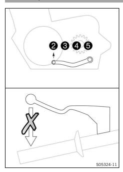
When the  $\underline{\text{quickshifter}}$  is activated, you can shift up without actuating the  $\underline{\text{clutch}}$ .
