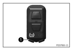
Press the TC button to switch traction control on or off.
