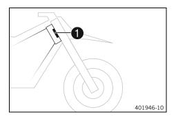
Frame label **1** is attached to the front of the steering head.
