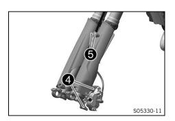
Position the brake caliper. Mount and tighten screws 4. Guideline
