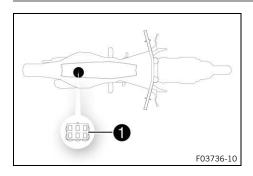
Diagnostics connector 1 is located under the seat.
