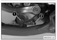
Mount and tighten screw plug 1 with the O-ring. Guideline
