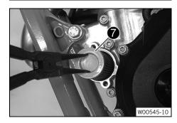
Pull oil filter out of the oil filter housing.
