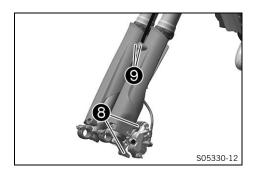
Position the brake caliper. Mount and tighten screws 8.
