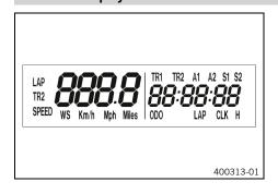
To enable you to check that the display is functioning properly, all display segments light up briefly.
