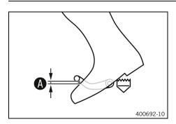
Sit on the vehicle in the riding position and measure the distance A between the upper edge of your boot and the shift
