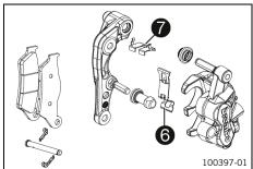
Check that spring steel clip 6 in the brake caliper and brake pad guide plate **7** in the brake caliper support are properly seated.
