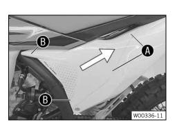
Condition: Air filter box cover not secured
