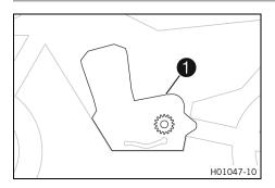
The engine number **1** is stamped on the left side of the engine above the front sprocket.
