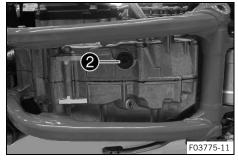
Mount and tighten screw plug 2 with new O-ring.
