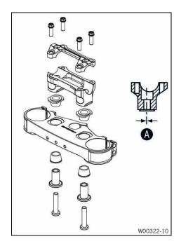
The holes on the handlebar support are placed at a distance of  $oldsymbol{\mathbb{A}}$  from the center.
