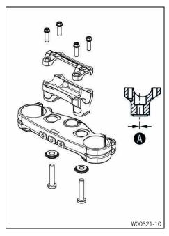
The holes on the handlebar support are placed at a distance of **A** from the center.
