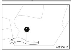
Brake pedal is located in front of the right footpeg. The rear brake is operated with the brake pedal.
