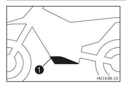
Remove screws 1 and engine guard.
