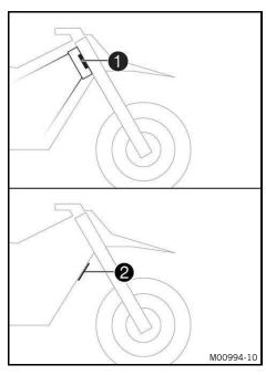
The type approval label 1 is fixed to the front of the steering head.
