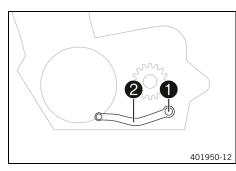
Remove screws 1 with the washers and remove gear shift
