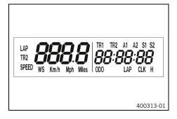
The combination instrument is activated when one of the buttons is pressed or an impulse comes from the wheel speed sensor.
