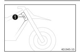
The vehicle identification number **1** is stamped on the bottom right of the frame behind the steering head.
