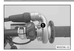
Stop button **1** is located on the right side of the handlebar.
