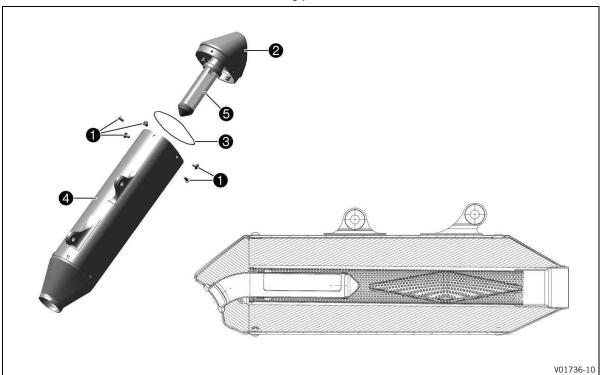
Remove screws 1 and take off silencer cap 2 with 0-ring 3.
