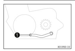
Gear shift lever 1 is mounted on the left of the engine.
