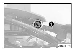
Ignition lock **1** is located to the right of the combination instrument.
