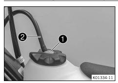
Mount the fuel tank filler cap and turn it clockwise until release button engages.
