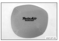
Mount the air filter water protection.
