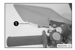
Clutch lever is fitted on the left side of the handlebar. The clutch is activated hydraulically and adjusts itself automatically.
