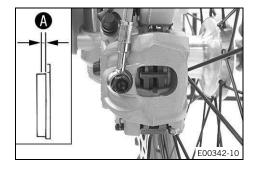
Check all brake pads on both brake calipers for their lining thickness .
