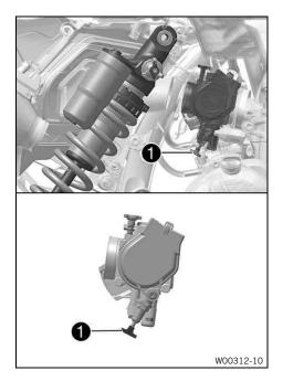
The cold start button **1** is fitted to the bottom of the throttle valve body.
