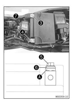
Connect positive cable 3 to the 12 V battery.
