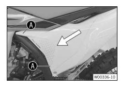
Condition: Air filter box cover not secured
