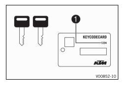
The key number **1** for the steering lock is stamped onto the key connector.
