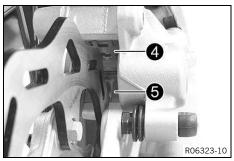
Check that spring steel clip 4 in the brake caliper and brake pad guide plate 5 in the brake caliper support are properly seated.
