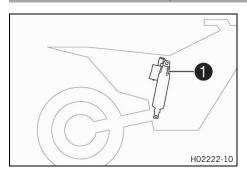
Shock absorber part number **1** is stamped on the top of the shock absorber above the adjusting ring towards the engine side.
