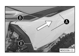
Condition: Air filter box cover secured
