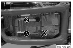
Remove screw plug 2 with O-ring.
