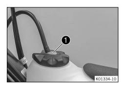
Press release button 1, turn the fuel tank cap counterclockwise, and lift it off.
