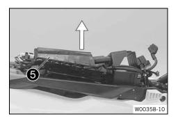
Pull up battery holding bracket 6 and remove the 12-V battery to the rear.
