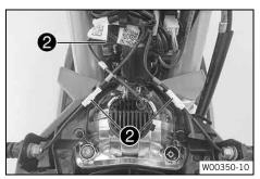
Detach plug-in connectors 2 and take off the headlight mask with the headlight.
