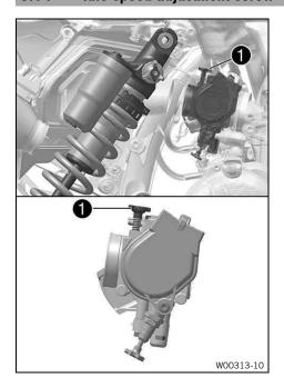
The idle setting of the throttle body substantially influences the vehicle's starting behavior, a stable idle speed, and the vehicle's response when the throttle is opened.
