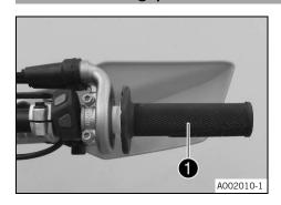
The throttle twist grip **1** is fitted on the right side of the handlebar.
