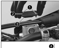
Correct the brake fluid level to level A.
