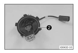
Insert the LED unit into the reflector and turn it clockwise all the way.
