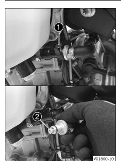
Clean quick-lock coupling 1 thoroughly with compressed air.
