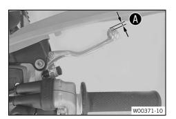
Push the hand brake lever to the handlebar and check free travel A.
