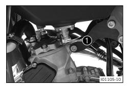
Using the tap handle ① on the fuel tap, you can open or close the fuel supply to the carburetor. The fuel tap is on the left side of the fuel tank.
