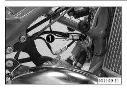
Plug-in connector **1** of the ignition timing map adjustment is located under the fuel tank in the cable compartment.
