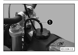
Mount the fuel tank cap and turn it clockwise until the fuel tank is tightly closed.
