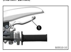
Hand brake lever **1** is fitted on the right side of the handlebar. The front brake is engaged using the hand brake lever.
