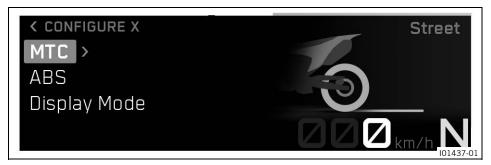
In the combination instrument, the motorcycle traction control can be switched on or off via the **MTC** submenu (optional).
