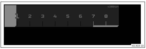
The engine speed is displayed in revolutions per minute.
