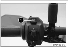
ABS button **1** is fitted on the left side of the combination switch.
