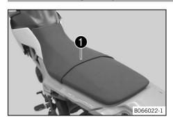
Supporting strap **1** is used for maneuvering the motorcycle. If you carry a passenger, the passenger can hold onto the grab handles during the trip.
