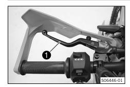
Clutch lever 1 is fitted on the left side of the handlebar.
