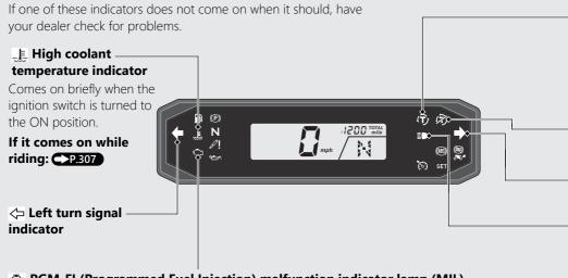
PGM-FI (Programmed Fuel Injection) malfunction indicator lamp (MIL)
