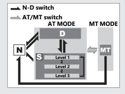
**Neutral (N):** Neutral is selected automatically when you turn the ignition switch to the ON position.
