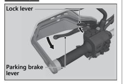
Place your vehicle on a firm, level surface. Stop the engine and push your vehicle while the parking brake is set to check the efficacy of the parking brake.
