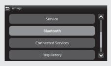
2 Select [Phone Pairing] or [Headset Pairing], and then press the **ENT** switch to enter the setting menu.
