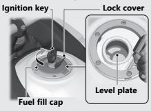
Do not fill with fuel above the level plate. Fuel type: Unleaded gasoline only Recommended fuel octane number:
