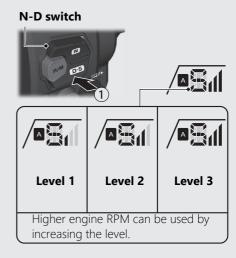
The selected level is maintained even when the ignition switch is turned to the OFF position, or transmission is switched to out of S mode.
