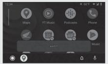
Push forward the **\**/<sub>|\lambda</sub> voice control switch on the left handlebar to operate **Android Auto**™ with your voice.
