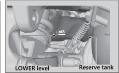
If the coolant level is dropping noticeably or the reserve tank is empty, you likely have a serious leak. Have your vehicle inspected by your dealer
