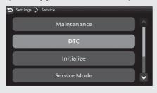
1 Select [DTC], and then press the ENT switch.
