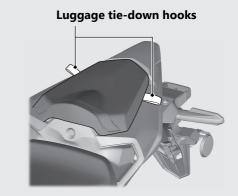
Never use the tie-down hooks to tow or lift the vehicle.
