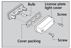
**3.** Install a new bulb and reinstall the parts in the reverse order of removal.
