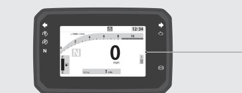
Do not operate the display functions for a long time with the engine stopped. It may result in a low (or dead) battery.
