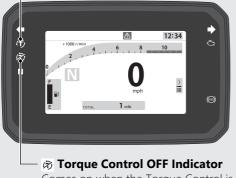
Comes on when the Torque Control is turned Off.
